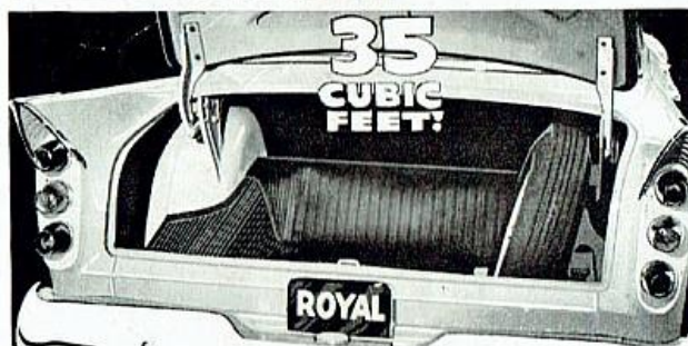
FAMILY-SIZE LUGGAGE BOOT. 35 cubic feet of space. Boot floor has rubber mat. Lid is counterbalanced.
