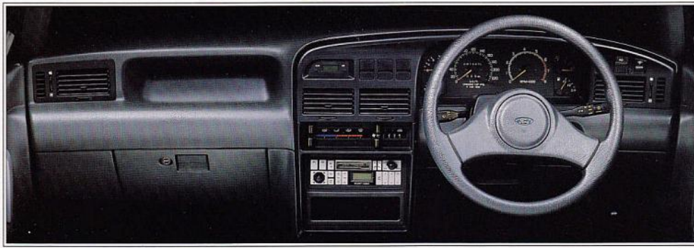
Ford Capri, full instrumentation, turbo model includes turbo boost gauge.
