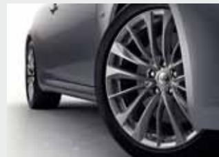
19 X 8.5-INCH ALUMINIUM-ALLOY WHEELS
