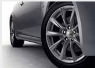
18 X 8.0-INCH ALUMINIUM-ALLOY WHEELS
