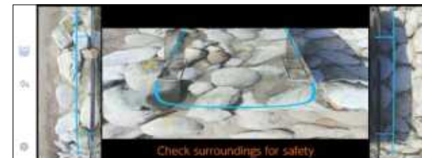
Underfloor View (Rear wheels) (Enlarged)
