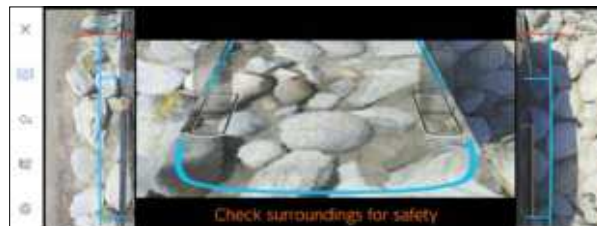
Underfloor View (Rear wheels) and Both-sides View
