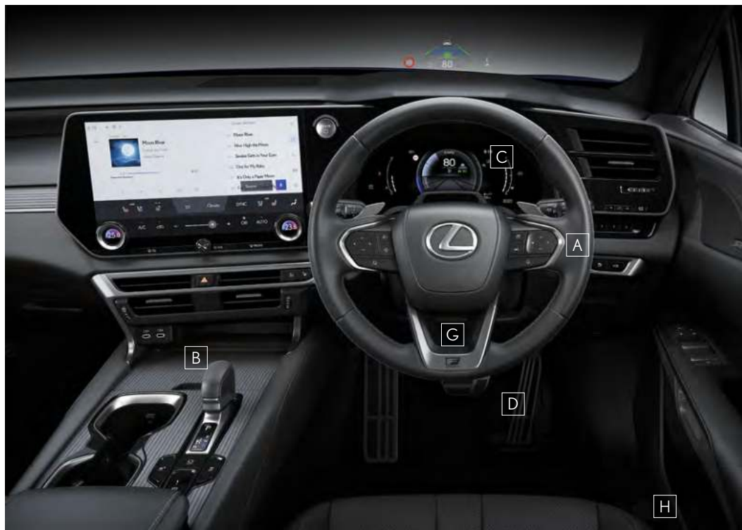
F SPORT Performance/F SPORT features A_Dimpled leather-accented steering wheel with paddle shifters / B_Dimpled leather-accented shift knob / C_TFT meter / D_Aluminium sport pedals and footrest / E_Real aluminium ornamentation / F_Leather-accented sport seats F SPORT exclusive features G_Emblem / H_Scuff plate
