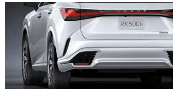
I_Rear lower bumper (Body-coloured)/Rear bumper molding (Piano Black)
