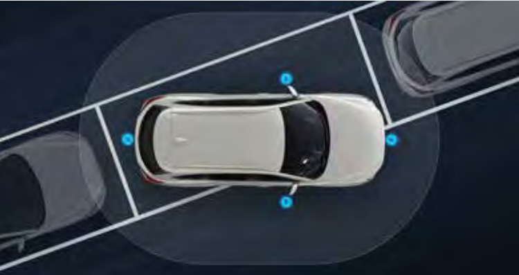
THE 360 VIEW MONITOR The 360° monitor employs four cameras to give you a complete aerial view of your surroundings so you can manoeuvre easily and safely!
