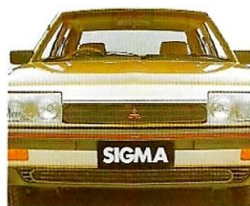
INSECT SCREEN: Easily installed or removed for cleaning, the screen prevents insects clogging the radiator or air-conditioning condenser.
