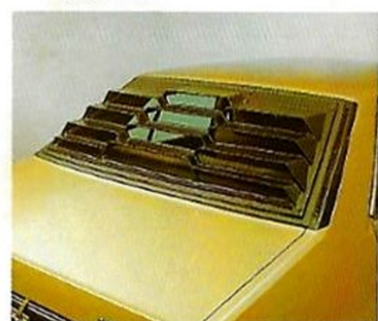
REAR WINDOW LOUVRE: Attractive and functional to protect the rear of the cabin from direct sunlight without hindering visibility.
