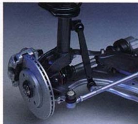
■ Front MacPherson type axle with stabilising bar : excellent steering and extreme course precision in bends.
