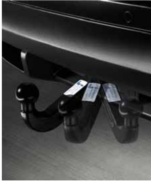
Towbar system with electrically deployable/retractable towball
