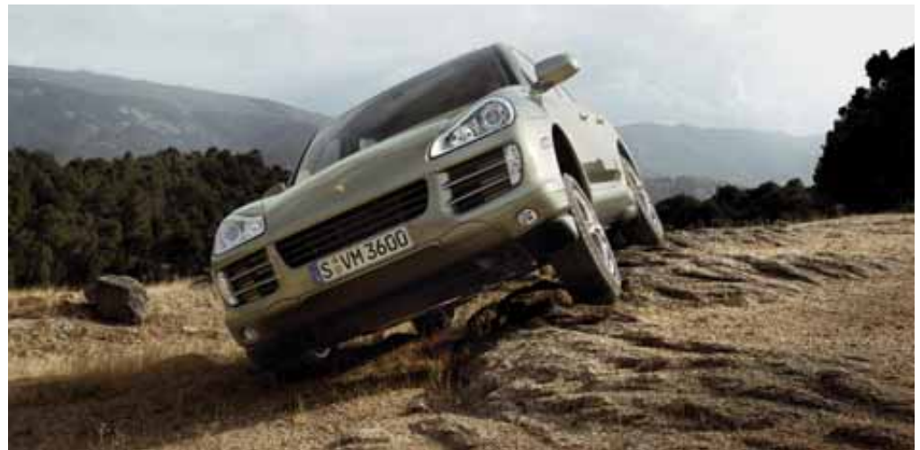
PDCC in off-road mode: increased wheel articulation
