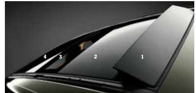
Panoramic roof system opened at rear
