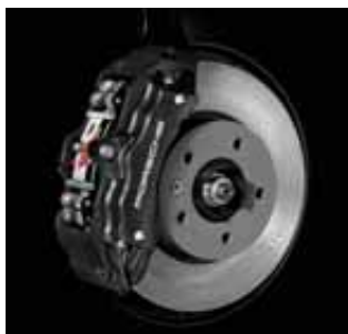
Cayenne: standard front brake with 330-mm disc
