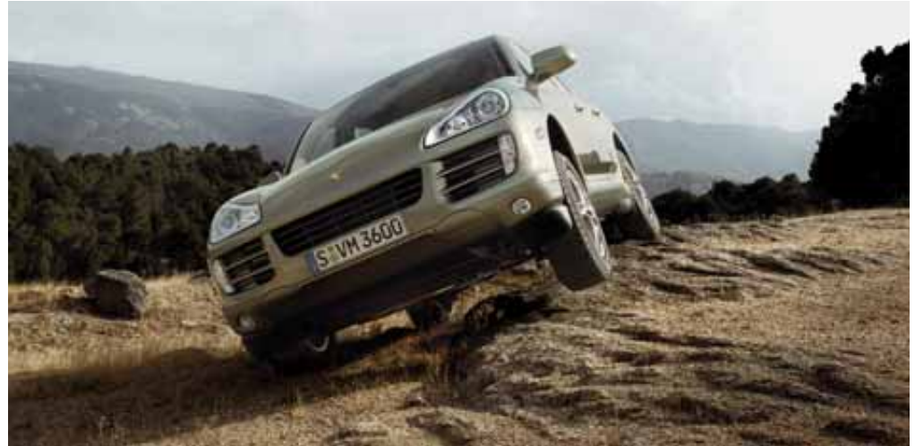
PDCC in on-road mode: reduced wheel articulation
