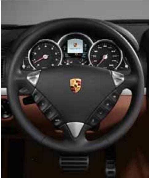
3-spoke multifunction steering wheel with Tiptronic S gearshift controls
