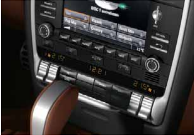
Air-conditioning controls (cover open)
