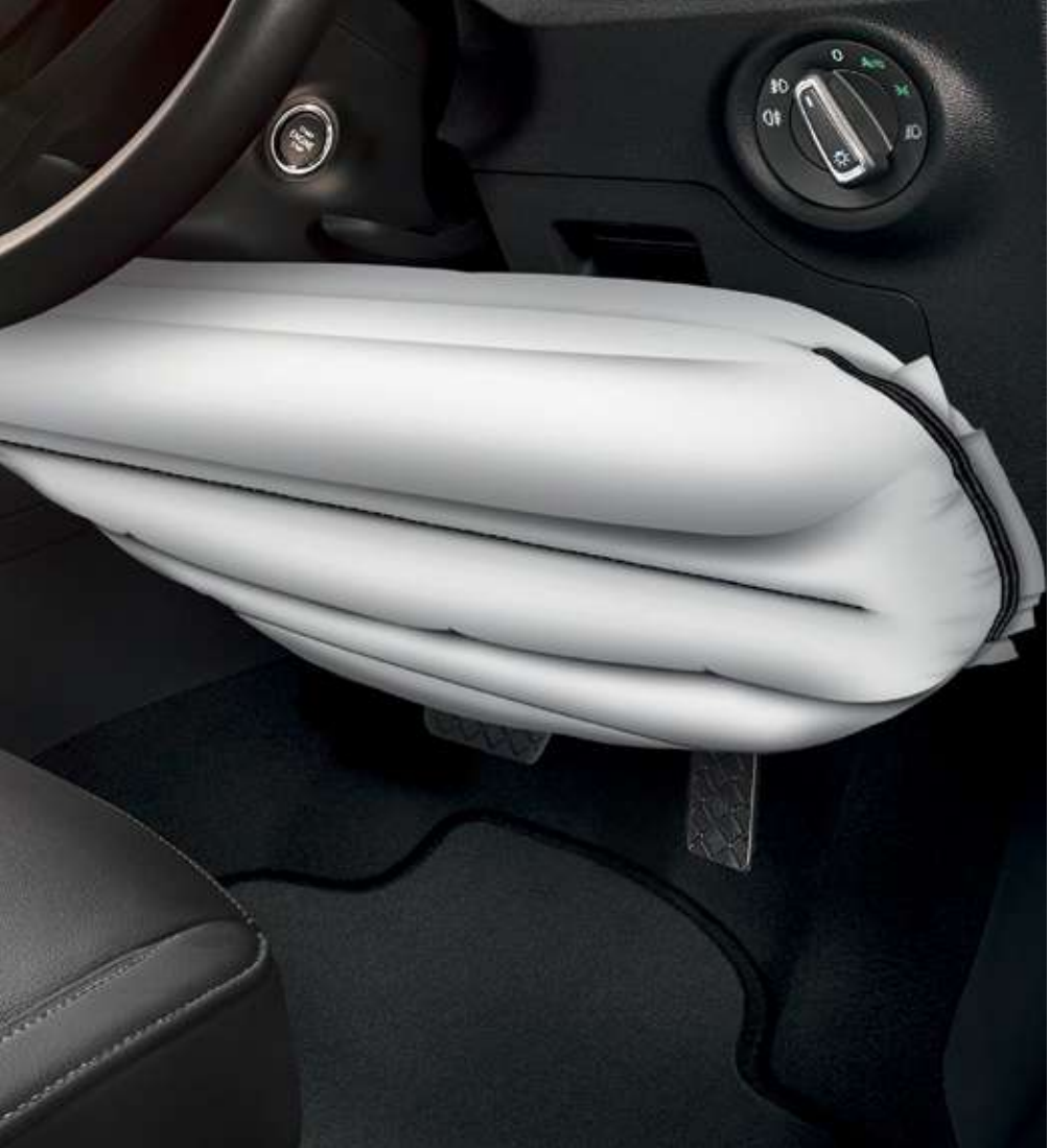
KNEE AIRBAG This airbag, which is located under the steering wheel column, protects the driver's knees and shins.
