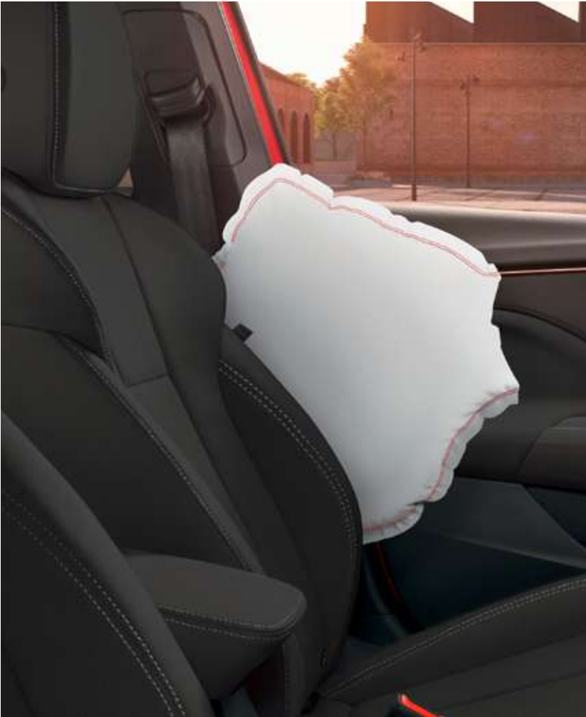
FRONT SIDE AIRBAGS These two airbags protect the pelvis and chest of the driver and passenger in the event of a side collision.
