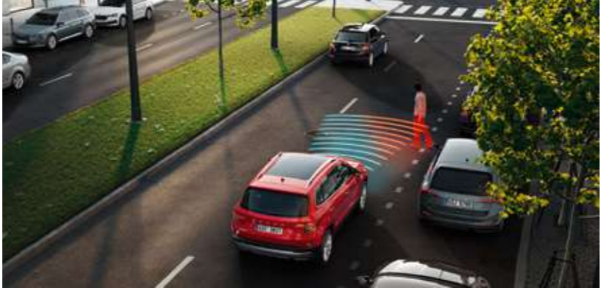
FRONT ASSIST WITH CITY EMERGENCY BRAKE o The Front Assist system, using a radar device in the front grille, is designed to monitor the distance from the vehicle ahead, including emergency braking function.
