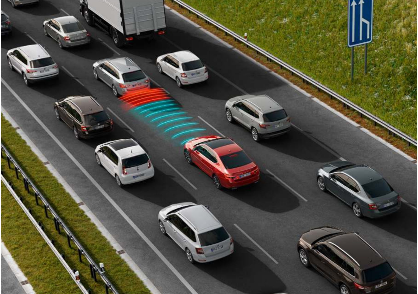
TRAFFIC JAM ASSIST / FOLLOW DRIVE This function is designed to facilitate driving in traffic jams. By controlling the engine brakes, and steering, it makes the vehicle pull away, brake, and turn to copy the movement of the surrounding vehicles (at speeds of up to 60 km/h). If lanes are not detected at speeds of up to 30 km/h, or only one lane (line) is detected at speeds of up to 60 km/h, the Follow Drive system follows the trajectory of the vehicle in front of you until lane markings are available again.
