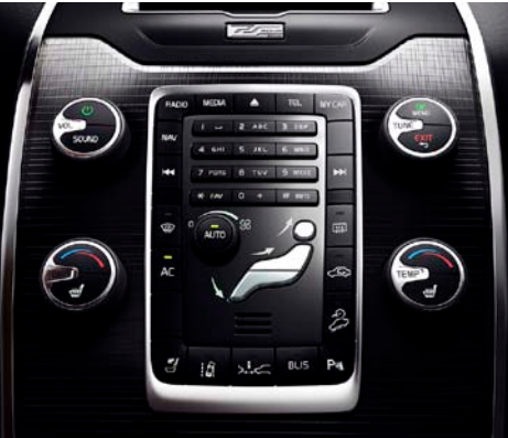
Electronic Climate Control (ECC)
