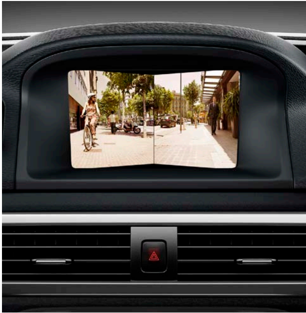
► Front blind view camera
