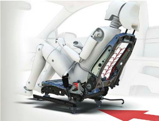
Whiplash Protection System (WHIPS)
