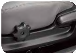
Driver's seat cushion tilt adjuster
