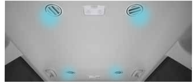
Roof Flushed 2 nd and 3 rd Row Diffused AC Vents
