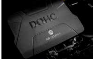
Kappa 1.2 MPI Engine The 83-ps, 1.2-liter dual-CVVT MPI engine with piston-cooling jets and coated piston rings is feisty and capable, yet also quiet and efficient.
