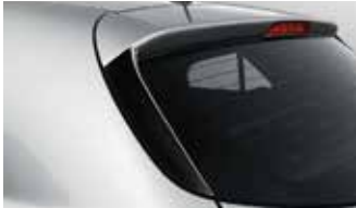
Rear spoiler garnish A rear spoiler improves the air vortex around the C-pillar for enhanced aerodynamics and downforce on the rear tires.
