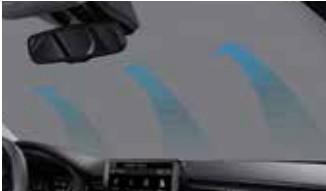
Auto defog system The auto defogger detects mist on the windshield and automatically deploys the fans to clear the glass rapidly.
