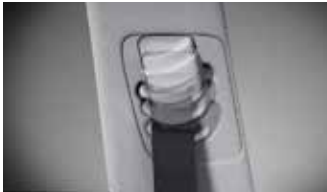
Adjustable seatbelt anchor The height-adjustable seatbelt anchors allow for seatbelts to be raised and lowered to achieve a perfect fit.
