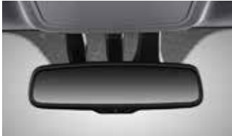
ECM rear-view mirror The Electro-Chromic Mirror automatically controls the glare from the headlamps of the car behind you at night.
