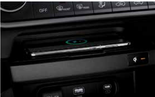
Wireless charging tray The charging pad in the dash, in front of the center console, lets you quickly charge compatible mobile phones, wirelessly.
