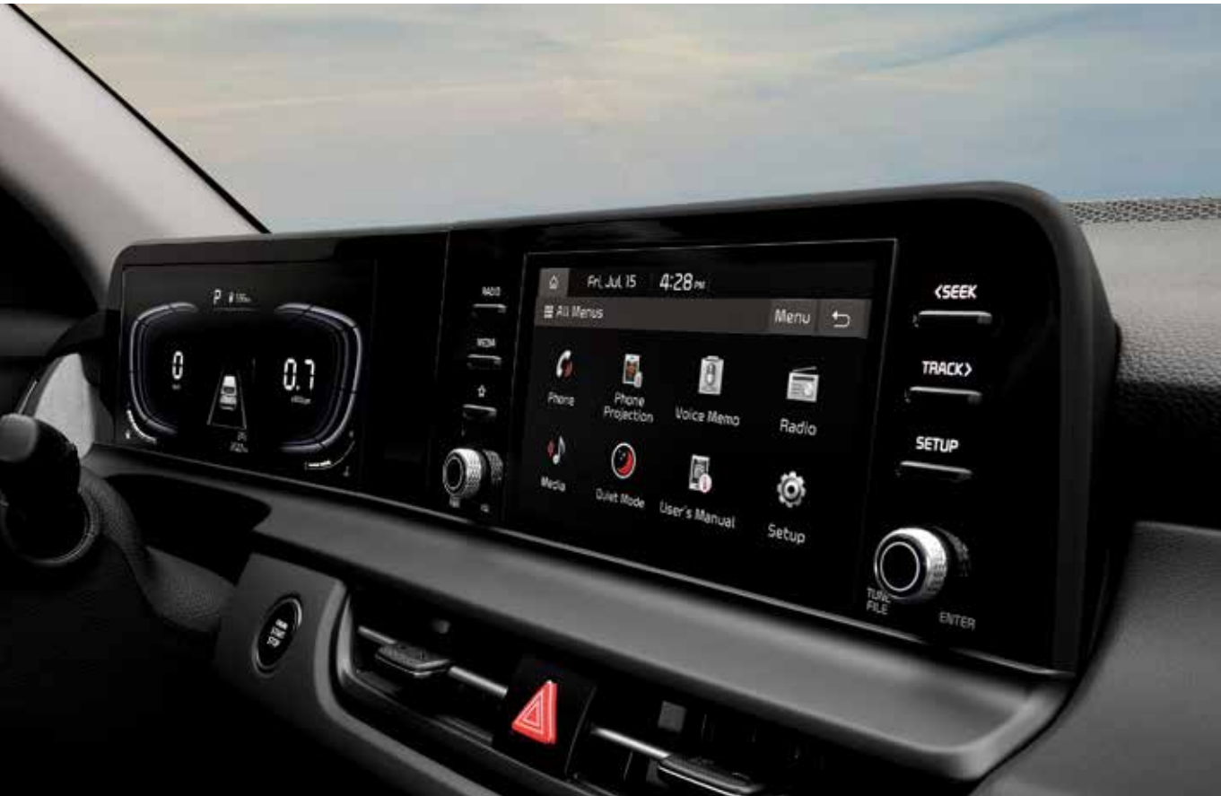
Panoramic curved display A gently curved instrument display sets a 4-inch platform cluster at the center, while to the side, a tasteful 8-inch audio display keeps entertainment data well organized and in clear view.
