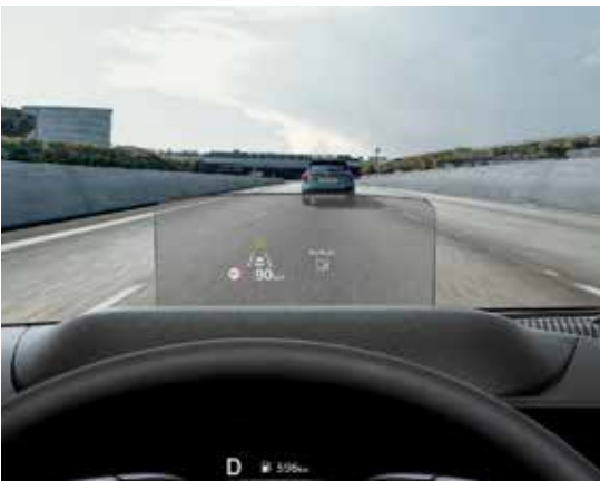
8-inch HUD The head-up display projects an image equivalent to an 8-inch screen onto the windshield. Your eyes stay on the road as you monitor speed, remaining distance to empty, cruise control, and DRIVE WISE technology data.
