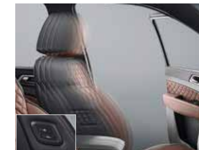
Passenger's seat walk-in device
