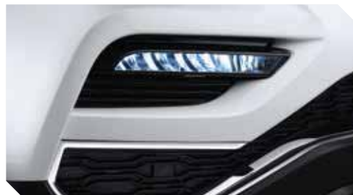
LED cornering light function combined with fog lamp
