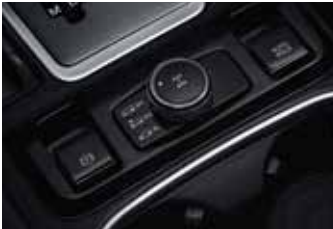
Electronic parking brake with auto-hold function
