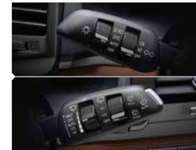
Headlamp control and automatic washer switches
