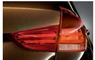
■ Adaptive Brakelights, two-stage, make it easier for drivers following from behind to see how hard you are applying the brakes. If you are applying the brakes in an emergency, the brakelights cover a larger area, allowing following traffic to distinguish between full application of the brakes and just a slight "tap" on the brakes. The result is an even higher standard of driving safety on the road.
