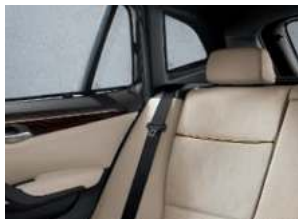
Sun blinds for the rear window and side windows of the rear compartment and luggage compartment.
