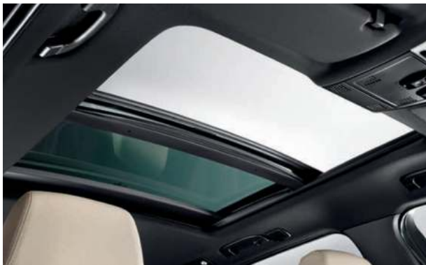
□ Panorama Sunroof with large opening and viewing area, plus wind deflector. The front half of the glass can be electrically raised by touch control and also has a sliding function, electric sliding roofliner, as well as a comfort open/close function with trap release.
