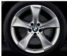
20" Star Spoke alloy wheels - Style 259 with run-flat performance tires. Front: 20 x 10.0 wheels with 275/40 tires; back: 20 x 11.0 wheels with 315/35 tires.
