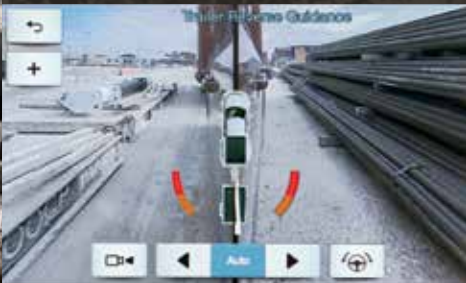
Trailer Reverse Guidance 1 automatically switches between side and rear camera views to show you what is most relevant while backing up your trailer, and provides overlays to guide you.
