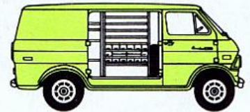
Service interior (any series or wb.) features bins, cabinets, shelves
