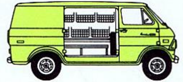
Utility interior (any series or wb.) features removable wire baskets
