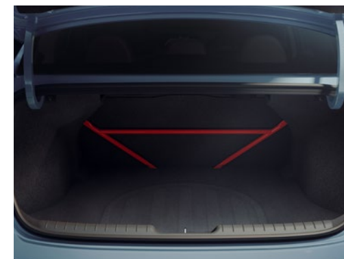
Rear strut bar offers an enhanced body rigidity increase of 29%, compared to the standard ELANTRA model
