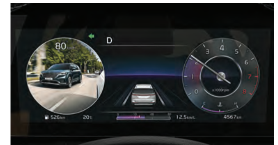
Blind view monitor 1 activates within the instrument panel when you turn on the blinker to change lanes, to display the blind spot in the direction of your turn signal.
