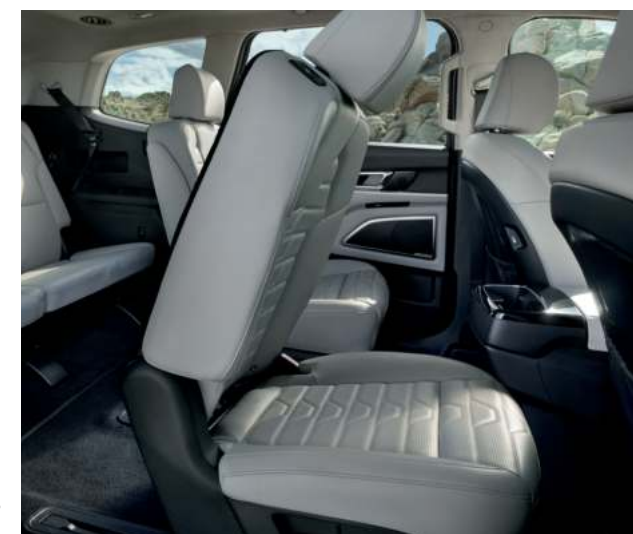
One-touch slide and fold 2 nd row seats to give 3 rd row passengers easy access.
