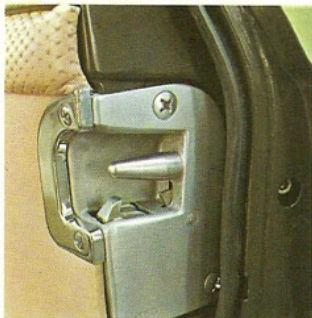
Safety-cone door locks are impregnable.
