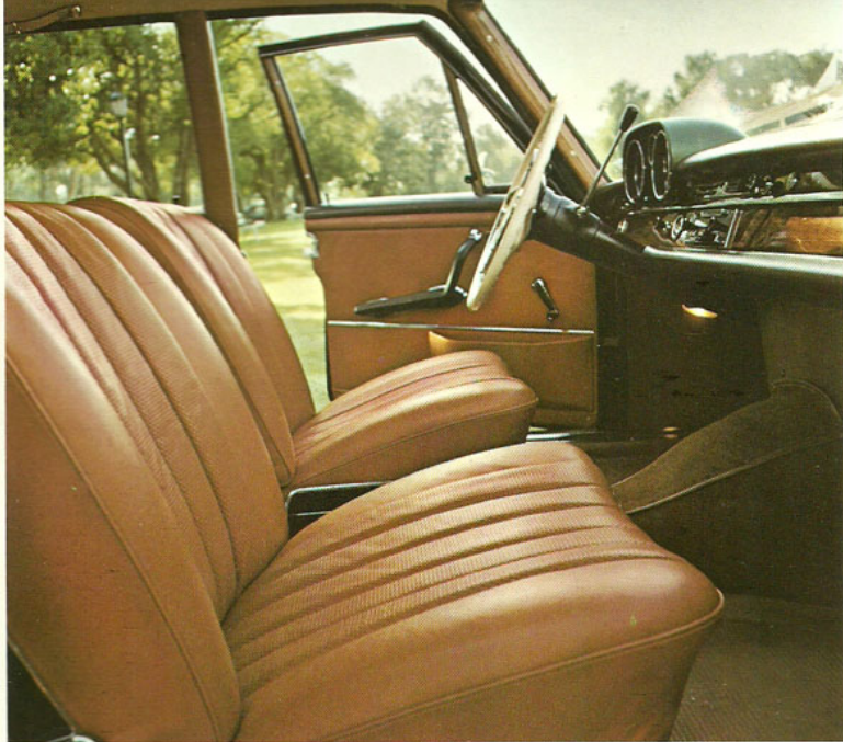
Pull a lever, front seats move up or down. Flick another lever, they roll fore and aft.
