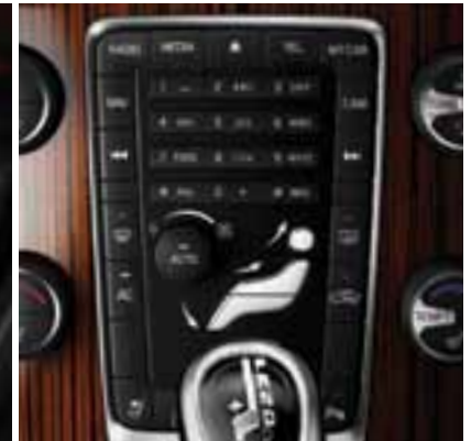
Electronic Climate Control (ECC)
