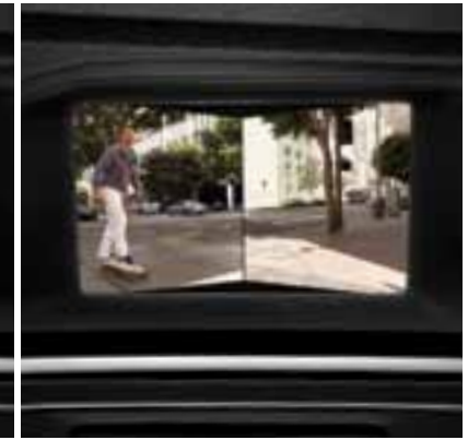
Front Blind View Camera
