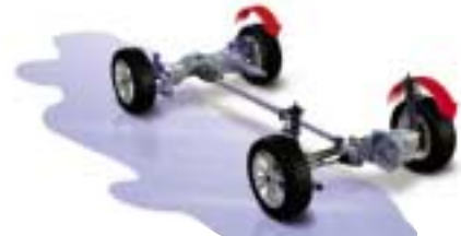
If one or both wheels on one side of the vehicle spin, more power goes instantly to the wheels with better traction.
