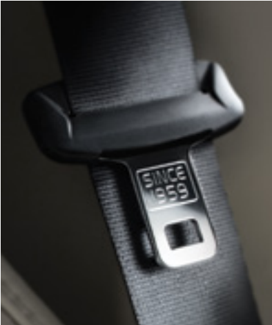
Prepared, seat belts tighten automatically if the car detects that a collision is likely, to ensure you're in the safest position should one occur.
