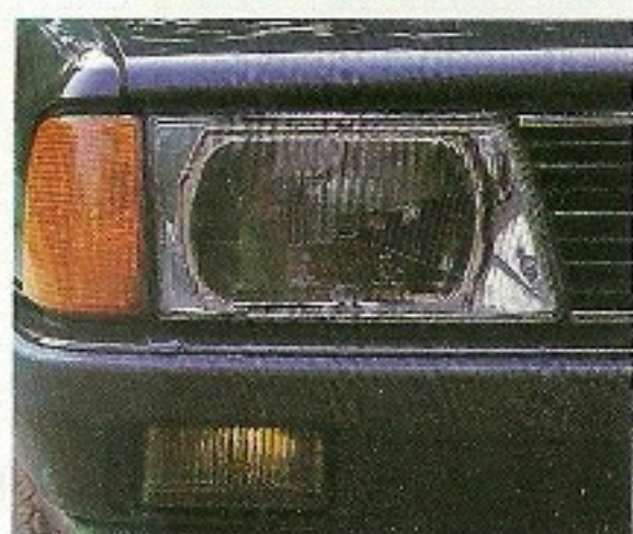
宽角度卤素灯 Wide rectangular halogen headlights.
