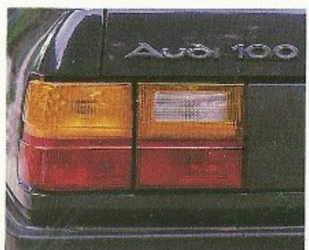
一体化后雾灯 Integrated rear fog light.
