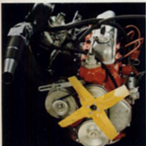
2 liters B 20-motor, 90, alternativt 118 hk SAE.
