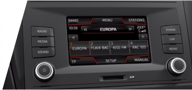
SEAT Media System Color (With AUX-IN, USB, SD Card Slot and 6 speakers)
