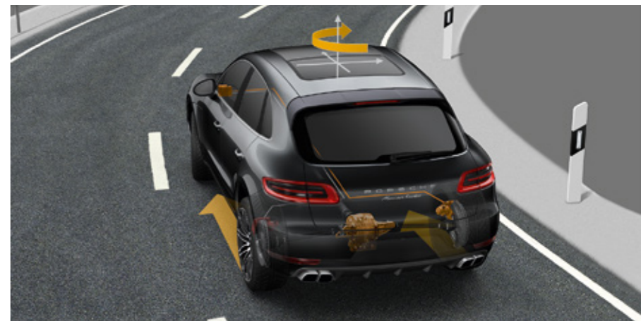
Porsche Torque Vectoring Plus (PTV Plus)
