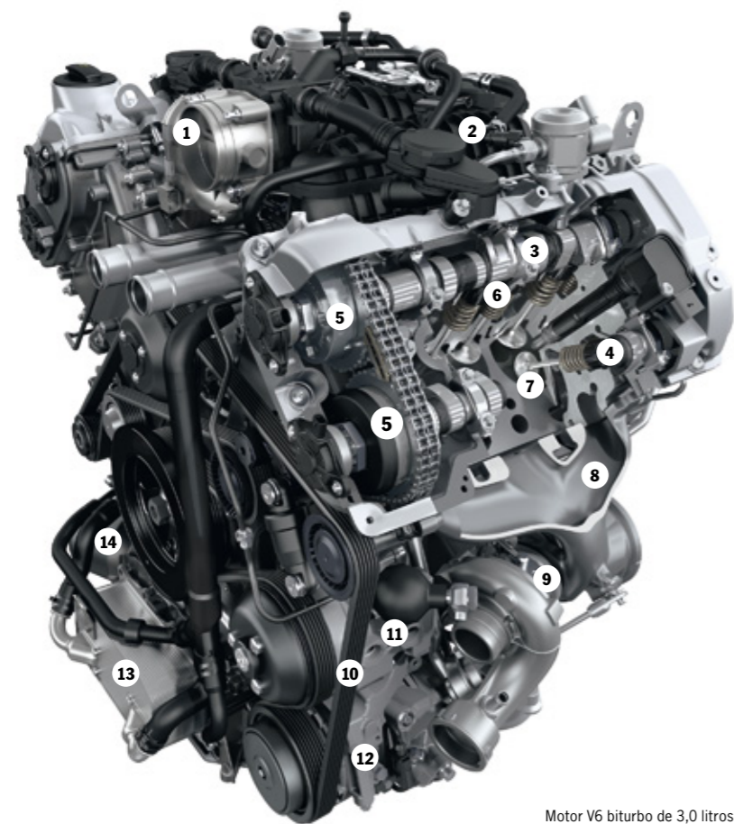
Motor V6 biturbo de 3,0 litros
