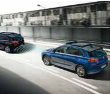
Advanced Smart Cruise Control (ASCC) maintains a pre-set distance to the preceding vehicle, automatically reducing or increasing speed as necessary.
