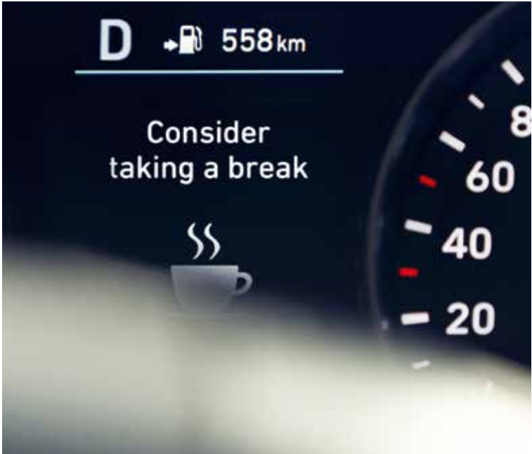
Driver Attention Alert (DAA) detects the onset of driver fatigue and provides both acoustic and visual alerts.
