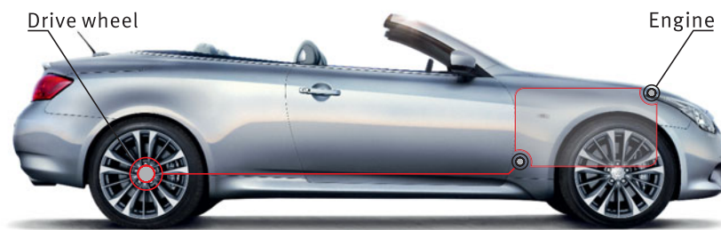
Rear-Wheel-Drive (RWD) and front mid-ship platform
