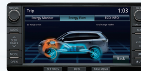
Energy flow indicator on MMCS
