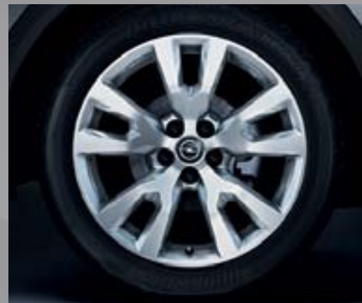
3 Alloy wheel, 7 J x 19, 5-V-spoke design, tyres 235/50 R 19
