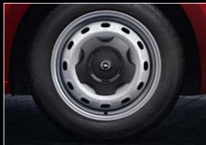
16" steel wheel with centre cap, 6 J x 16" (P91), tyres 205/65 R 16 1 .
