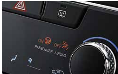
Front Passenger air bag ON/OFF indicator The front passenger air bag can be deactivated by switch if a child restraint is installed on the front passenger's seat.
