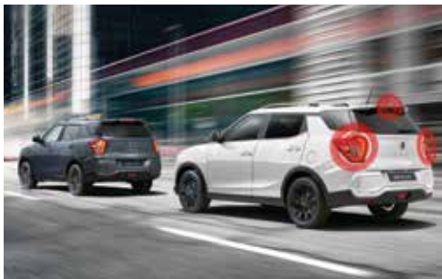
Emergency Stop Signal (ESS) During hard braking, ESS automatically activates the emergency flashers to warn drivers behind.
