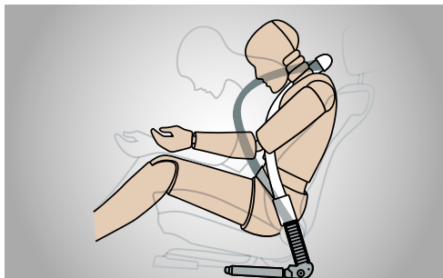
Safety belt dual pretensioner Pre-tensioning mechanism greatly reduces the risk of serious injury.
