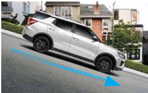
Hill Descent Control (HDC) Activating HDC on extremely steep hills automatically shifts the vehicle into lower gear and begins brake pumping action for a safe descent.
