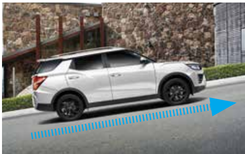
Hill Start Assist (HSA) On releasing the brake pedal while starting on a steep hill, HSA will maintain braking pressure until the throttle is applied thus preventing the vehicle from rolling backwards.
