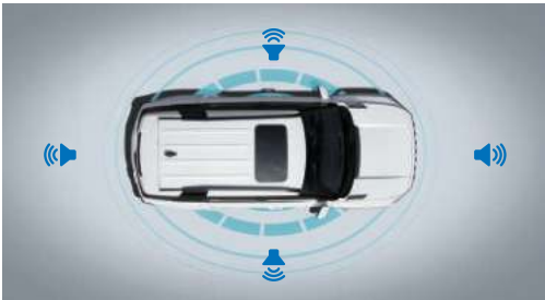
Virtual Engine Sound System (VESS)
