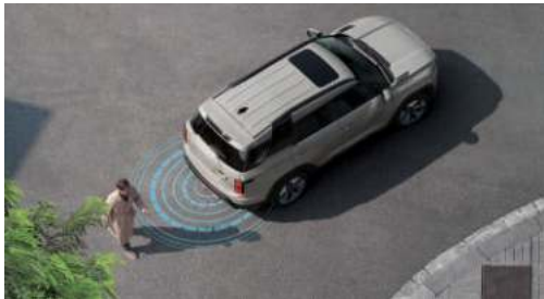
Acoustic vehicle alert system (AVAS) when reversing
