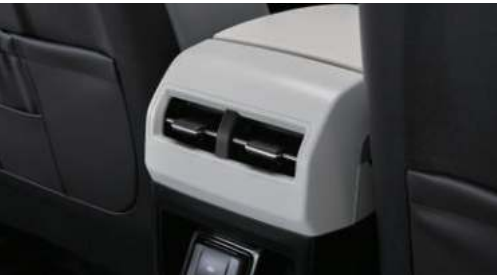
Rear centre console air vent
