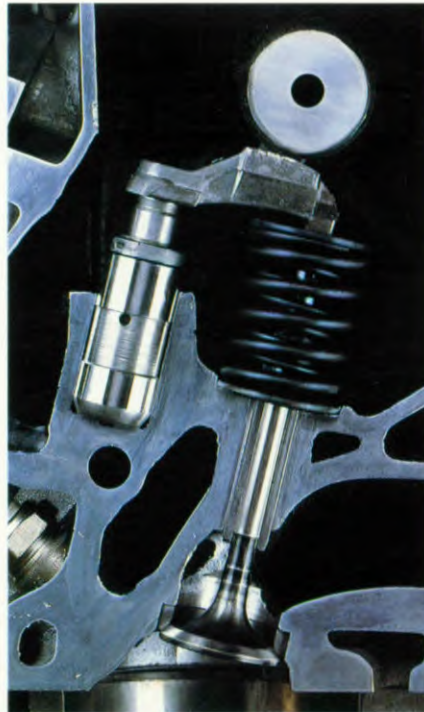
Valve lash adjuster
