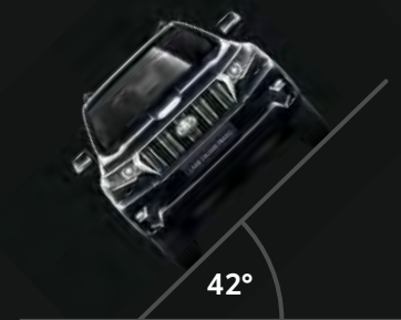
Limit angle of vehicle turnover
