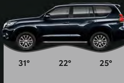
Approach, ramp break-over and departure angles
