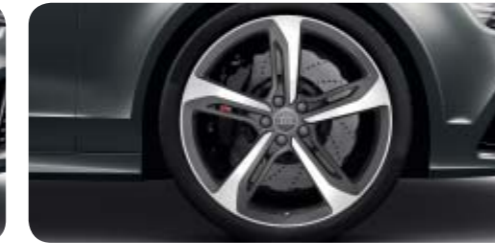
Cast aluminium wheels in 5-spoke blade design in matt titanium look, gloss turned finish 1 size 9 J x 21 with 275/30 R 21 tyres 2
