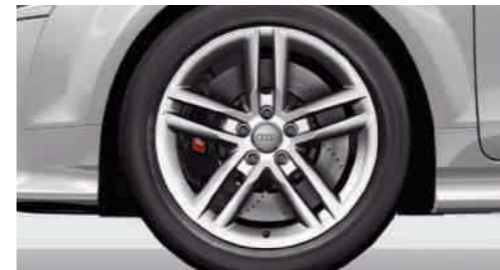
Cast aluminium wheels, 5-double-spoke design, size 9 J x 18 with 245/40 R 18 tyres
