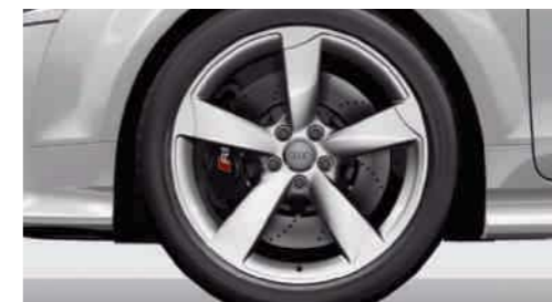
Cast aluminium winter wheels, 5-arm rotor design, size 9 J x 19 with 255/35 R 19 winter tyres, cannot be fitted with snow chains, permissible top speed 240 km/h
