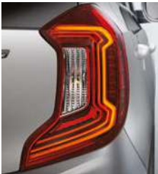
LED-type rear combination lamps*
