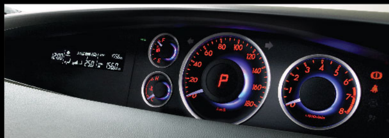
儀表組合位於向駕駛者的儀表板上方，把注意力被分散到路面以外的情況減至最低。 The broad meter cluster is located at the top of the dashboard towards the driver to minimize eye movement away from the road.
