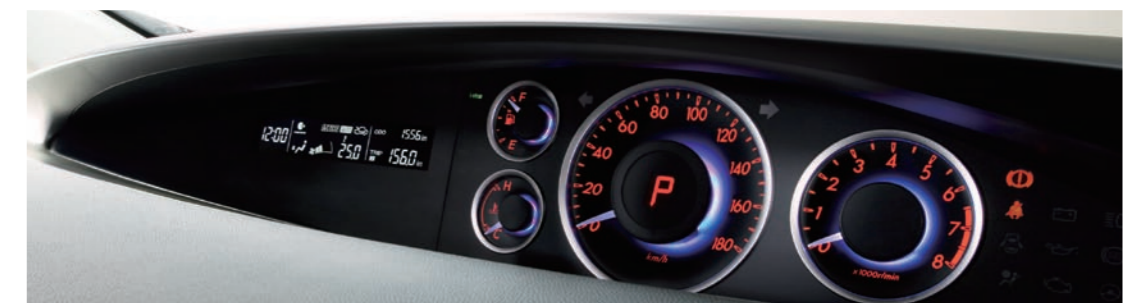
The broad meter cluster is located at the top of the dashboard towards the driver to minimize eye movement away from the road.
