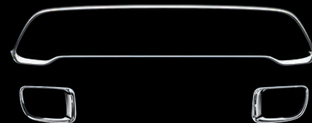
In addition to the radiator grille, chrome-plated air ducts for cooling the brakes.
